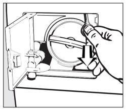
■ To open the door, pull down on the ring in the upper right corner of the access area.
